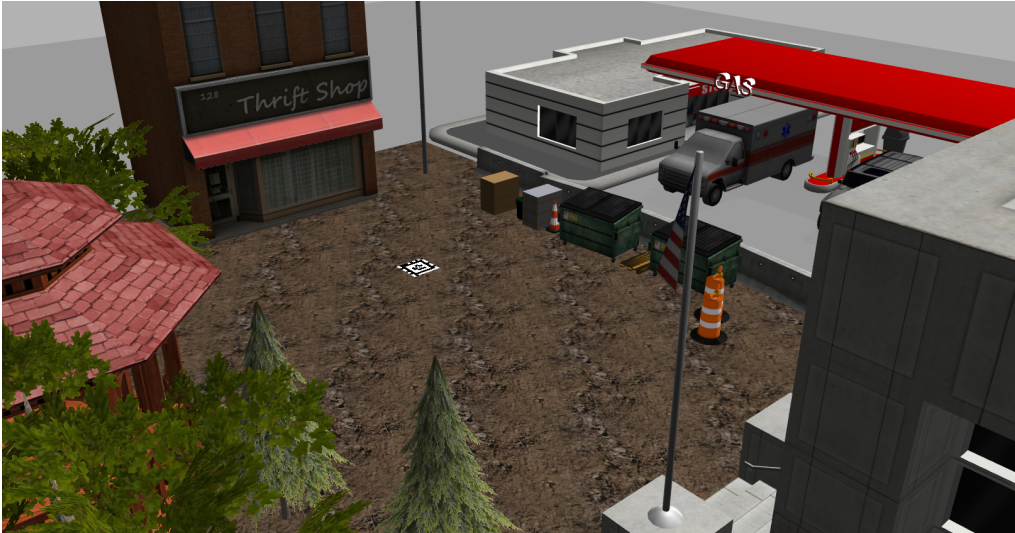
Figure 5.1: Gazebo world simulation. Note the AprilTag marker which is used as the landing pad.
