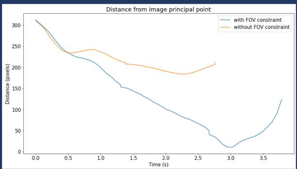
We can see that the FOV constraint allows the projected landing pad center to get closer to the principal point when compared to the same trajectory without FOV constraints.
